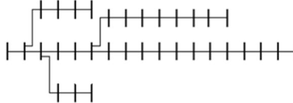
**Fig. 10:** The 33 bus radial distribution system.
