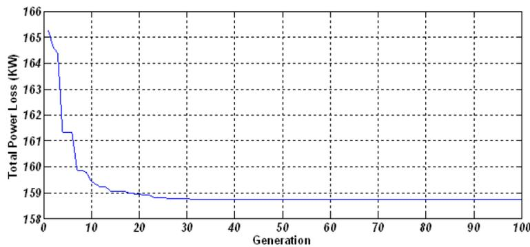
**Fig. 11:** Convergence characteristic of the 33 bus test system.
