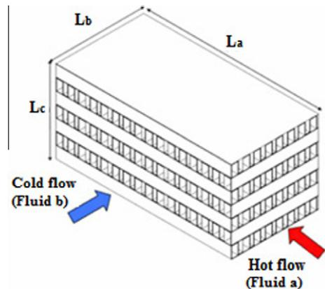
Fig. 1. Schematic representation of cross-flow plate-fin heat exchanger [18].
