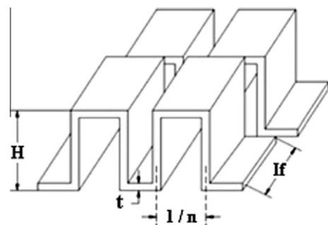
Fig. 2. detailed view of offset-strip fin [18].
